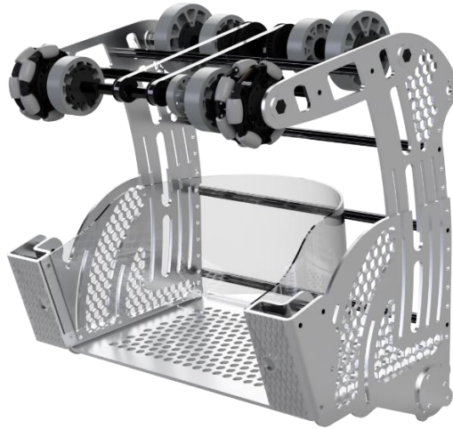
Front view of the grabber with the polycarbonate back guard visible
